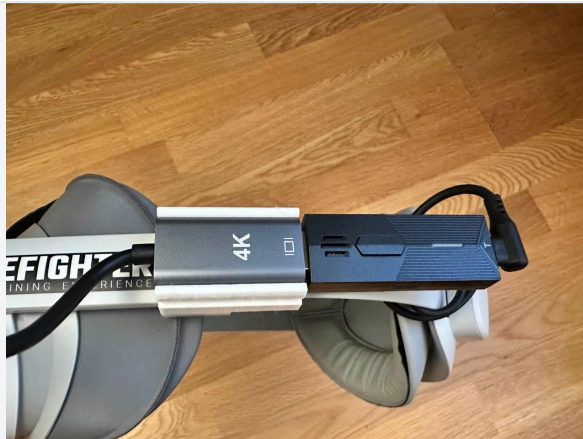
USB-C on HDMI Adapter, transmitter T and receiver R
