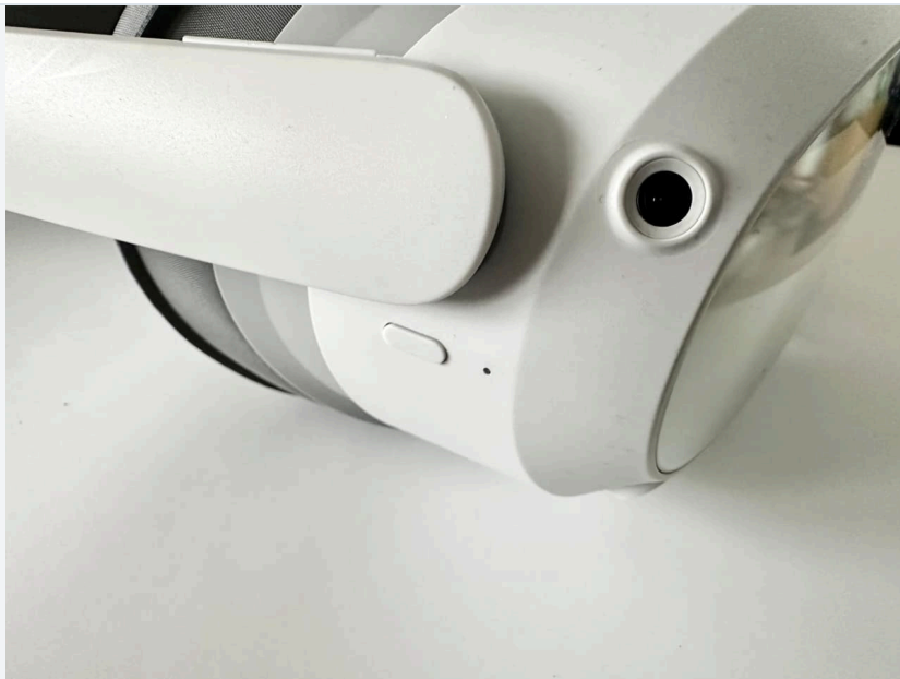
Position of the power button and status LED
